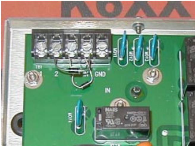
Photo 2. Diodes necessary inside the StackMatch for the single-wire two-stack controller
