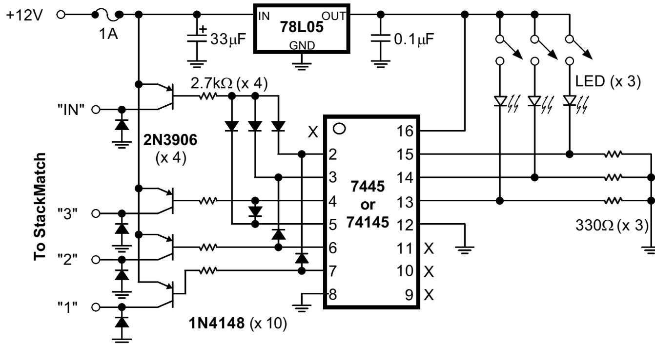
Figure 2. Three-Stack Controller using PNP output Transistors.
