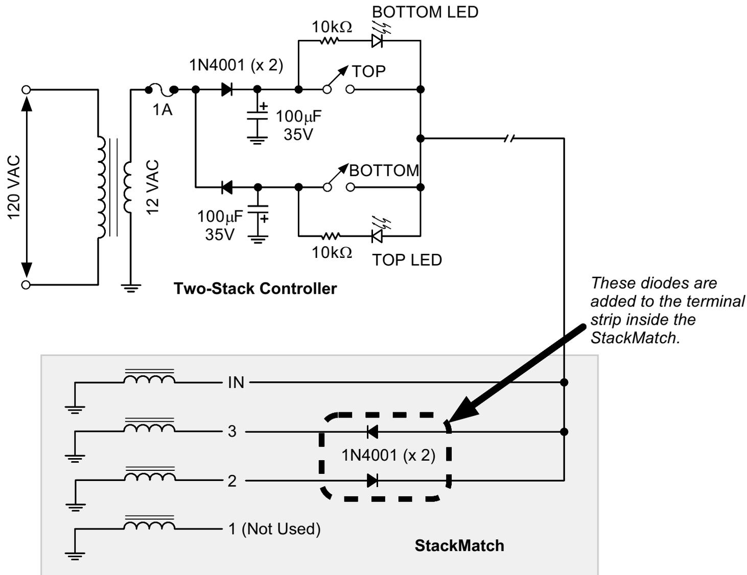
Figure 4. Two-Stack Controller and Additional Diodes Needed Inside the StackMatch.
