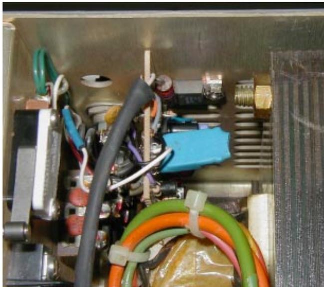
Photo 4. The board is installed on the rear panel between the power transformer and the tube compartment.
